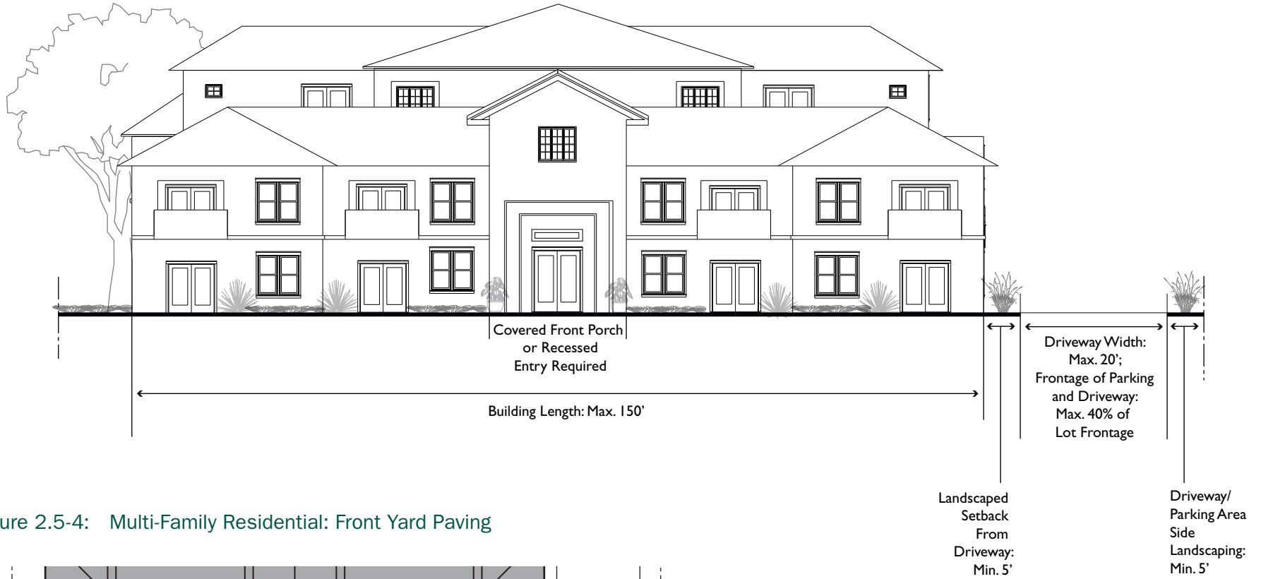
Figure 2.5-3: Multi-Family Residential: Elevation
