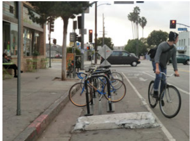
Example of Advanced Stop Bars. At a Signalized Intersection, the Bicyclist will Stop Ahead of Vehicles. Advanced stop bars allow for safer stopping and Starting While on a Bicycle, and Keep the Bicyclist Within Sight for all Auto Drivers.
