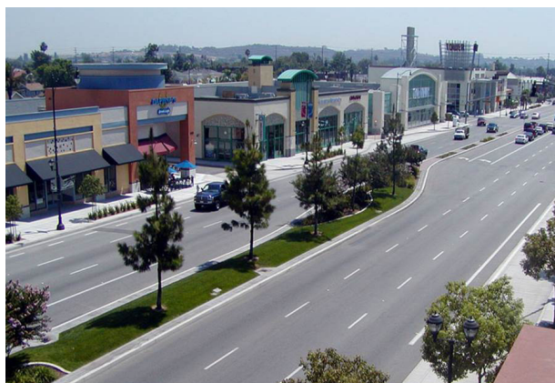
Example of how a Raised Median can Reduce Crossing Distance and Improve the Appearance of the Streetscape.
