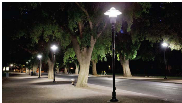
Pedestrian-Scaled Lighting- Shorter Poles Which Serve to Primarily Light the Sidewalk - Improve Visibility, and Sense of Security.
