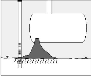
When installed and operated according to the manufacturer's instructions, a groundwater monitoring system meets the federal leak detection requirements for USTs. Operation of a groundwater monitoring system at least once each month fulfills the requirements for the life of a tank. Groundwater monitoring can also be used to detect leaks in piping (see the section on leak detection for piping starting on page 22).
