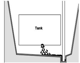
There are a number of interstitial monitoring methods. These methods include the use of a simple dipstick or a continuous, automated vapor or liquid sensor permanently installed in the system to monitor interstitial spaces. Interstitial spaces can also be filled with brine or glycol solutions and their levels monitored. Also, sophisticated pressure/vacuum monitoring systems may be used to indicate pressure changes within these spaces.
